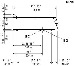
EI = Electrical inlet (power) **EQ** = Equipotential screw
