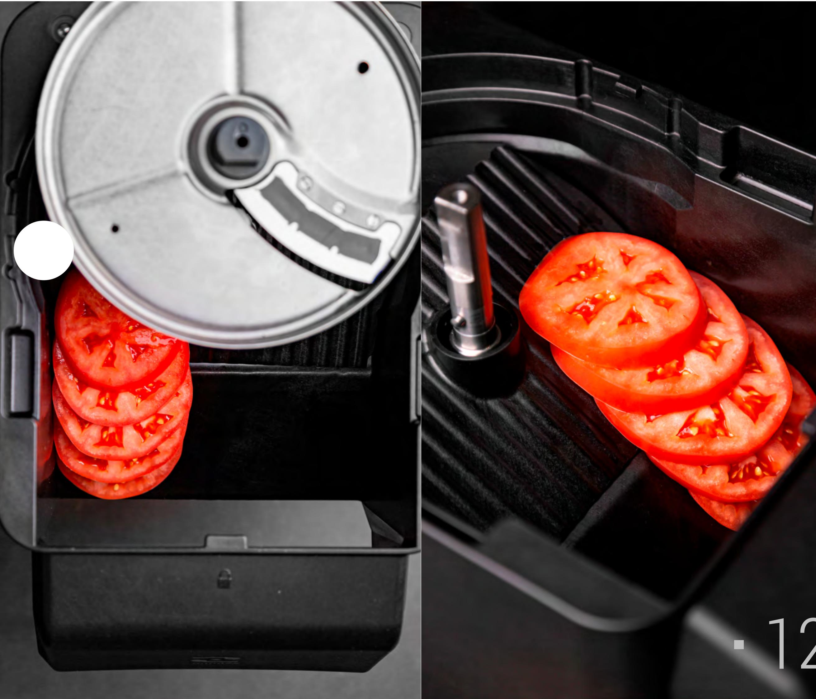
The ejection slide allows the cut product to be ejected by gravity, avoiding impacts. This feature is particularly useful for cutting slices and reconstructing the product for subsequent preservation or presentation.
