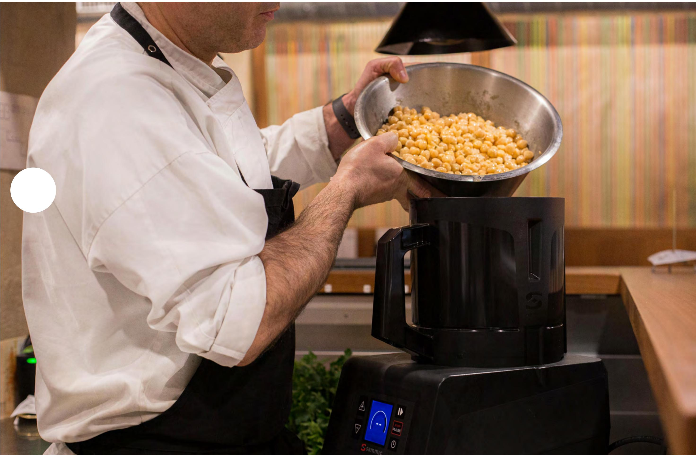
The K/KE food processors and CK combis are available with a 4.4 litre capacity bowl equipped with a high pipe and can grind, mix, knead... 2.5 kg of product, in seconds.
