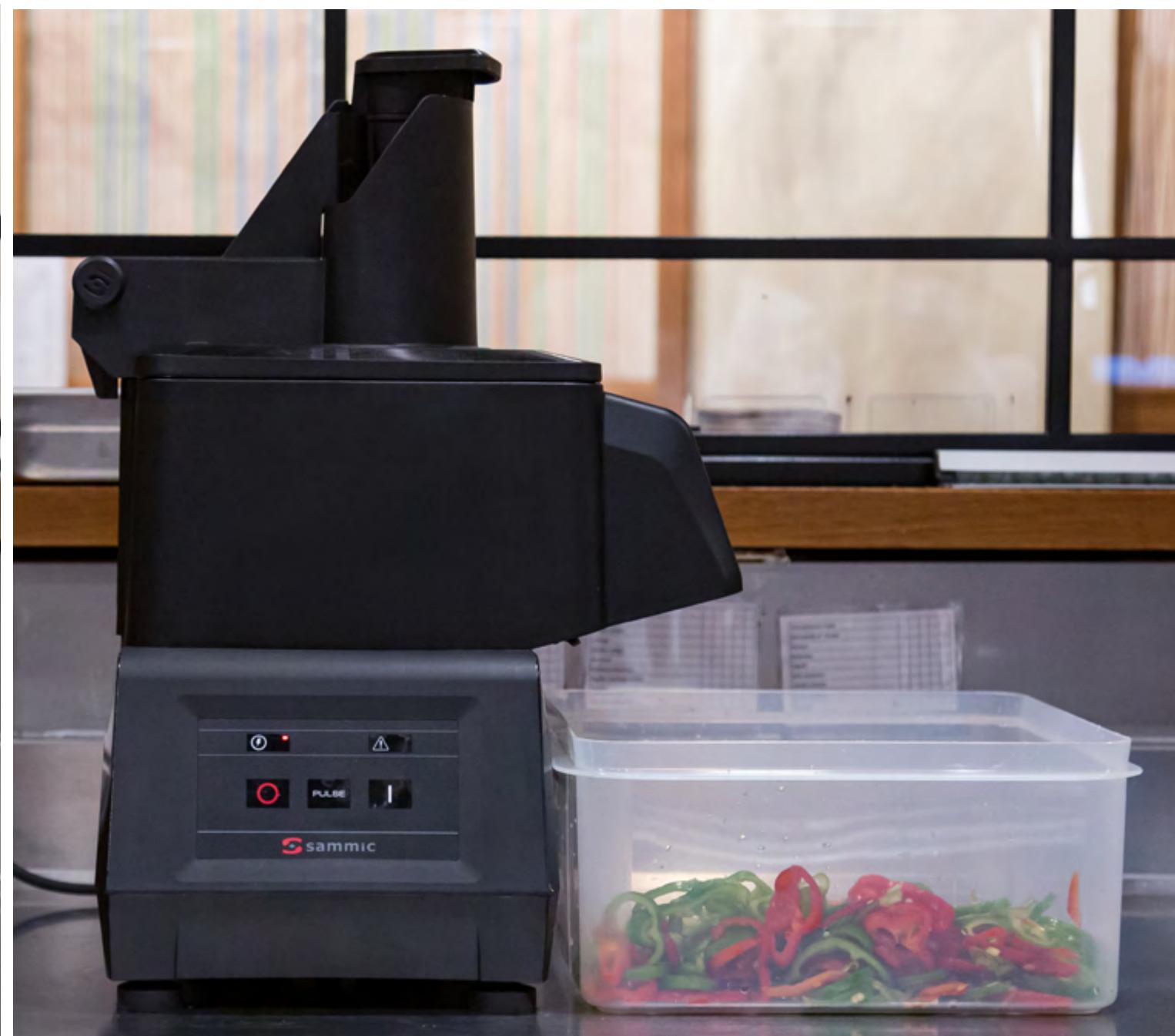
The design of the veg prep machine allows the product output to be positioned to the right or to the left depending on the user's needs at any given moment.
