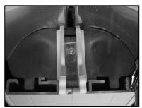
1. Using gentle force, push the lamp so that the sprung terminal pin and lamp end are compressed about 4mm, rotate alternate end of lamp up into the terminal block taking care to line up Centre Pin of Lamp with Terminal Pin in terminal block. Release spring and allow lamp to seat between the two terminal blocks. Jiggle lamp slightly to make sure it is secure in place.
