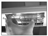
3. If replacing existing lamps, remove old lamp by gripping around large diameter of ceramic end. Using gentle force, push the lamp to one side so that the opposite end is clear of the Terminal Pin. Rotate lamp down and remove from heat lamp body.
